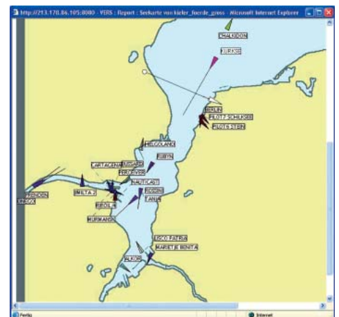
AIS based traffic picture from Kiel Fjord with passage condition, recorded by VERS
